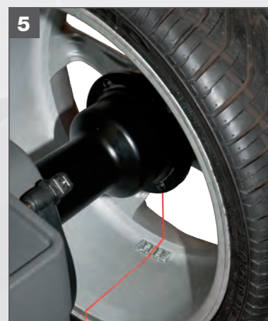
LASER LINE SYSTEM
