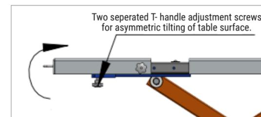
Two separated T-handle adjustment screws for asymmetric tilting of table surface.
