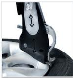
Suitable for Patented **QX Leverless** mounting device for low profiled and UHP tyres (optional).
