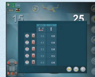
AAM for each single wheel, this software acquires wheel weight and size to recalculate the tolerance value and eliminate any perceived vibrations on the steering wheel. It guarantees the utmost comfort in driving the vehicle and, together with OW, minimizes the balancing time and wheel weights needed.
