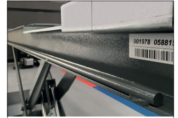
Includes sliding guide for Jacking Beams.
