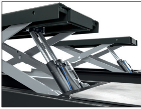
Lift and built in lifting table with double hydraulic circuit (2 masters + 2 slaves). Hydraulic security .
